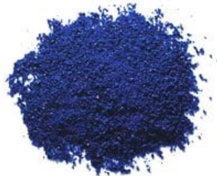
Glass frit is specially formulated to produce the distinctive cobalt blue AQUASTORE® glass coating.
